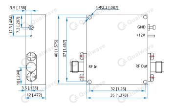
(The bottom of the amplifier needs to be equipped with a heat sink to assist in heat dissipation.)
