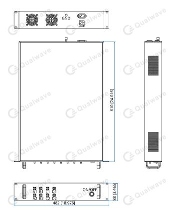
Unit: in[mm] Tolerance: ±0.2in [±0.008mm] \*This is a draft outline, which may be changed.
